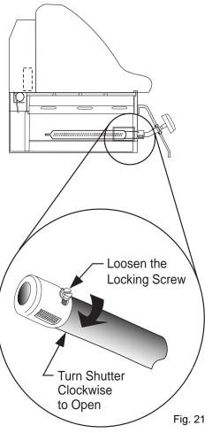
If burners are removed for cleaning or adjustment, always confirm that they have been reinstalled correctly over the valve outlets (see Fig. 22). The valves should extend into the burner venturis approximately 1/4".
